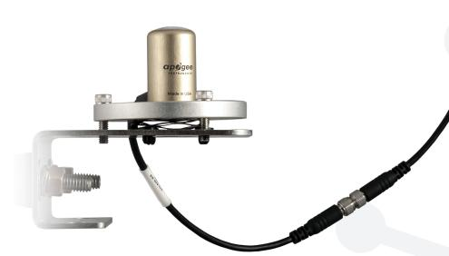
allows measuring of photosynthetic active radiation. it helps determine the amount of light the plants are exposed to.
